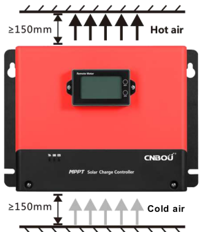
Fig. 2.1 Installation and Heat Dissipation
